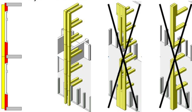
FIGURE 1: LEFT: FAÇADE INTERSECTION WITH ADDITIONALLY MOUNTED MODULES, RIGHT: DISCUSSED VENTILATION DUCTWORK INSIDE THE FAÇADE ELEMENTS
