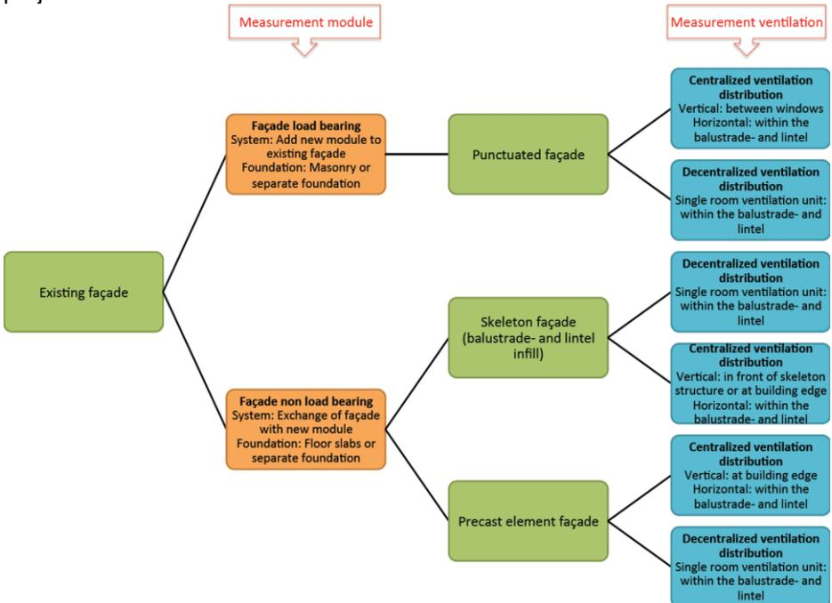
FIGURE 5: LINK BETWEEN TYPOLOGY AND CONSTRUCTION/VENTILATION
